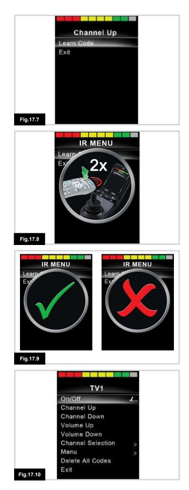
Select Learn Code, by using the Right button while the Command is highlighted, Fig 17.7.
