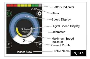
This is a typical screen. Depending on SID type, programing or system configuration and status, there may be additional icons.
