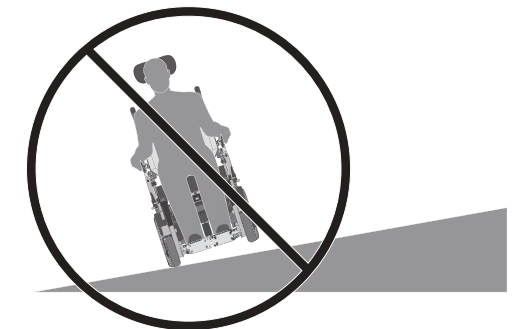
Figure 4. Do not turn on a slope.
