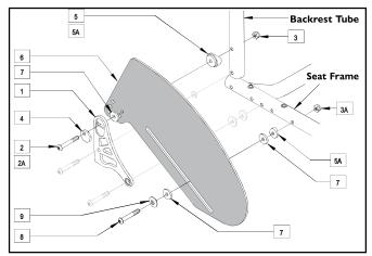
Figure A - Folding Back, Zero Offset
