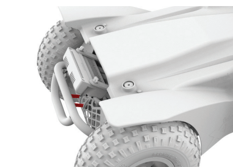
Figure 4.6b Extreme X8 brake levers released
