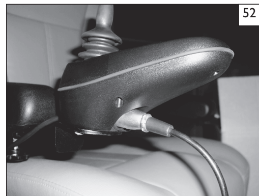
Off-board charger port located under joystick
