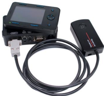
Connecting the Link to Omni
